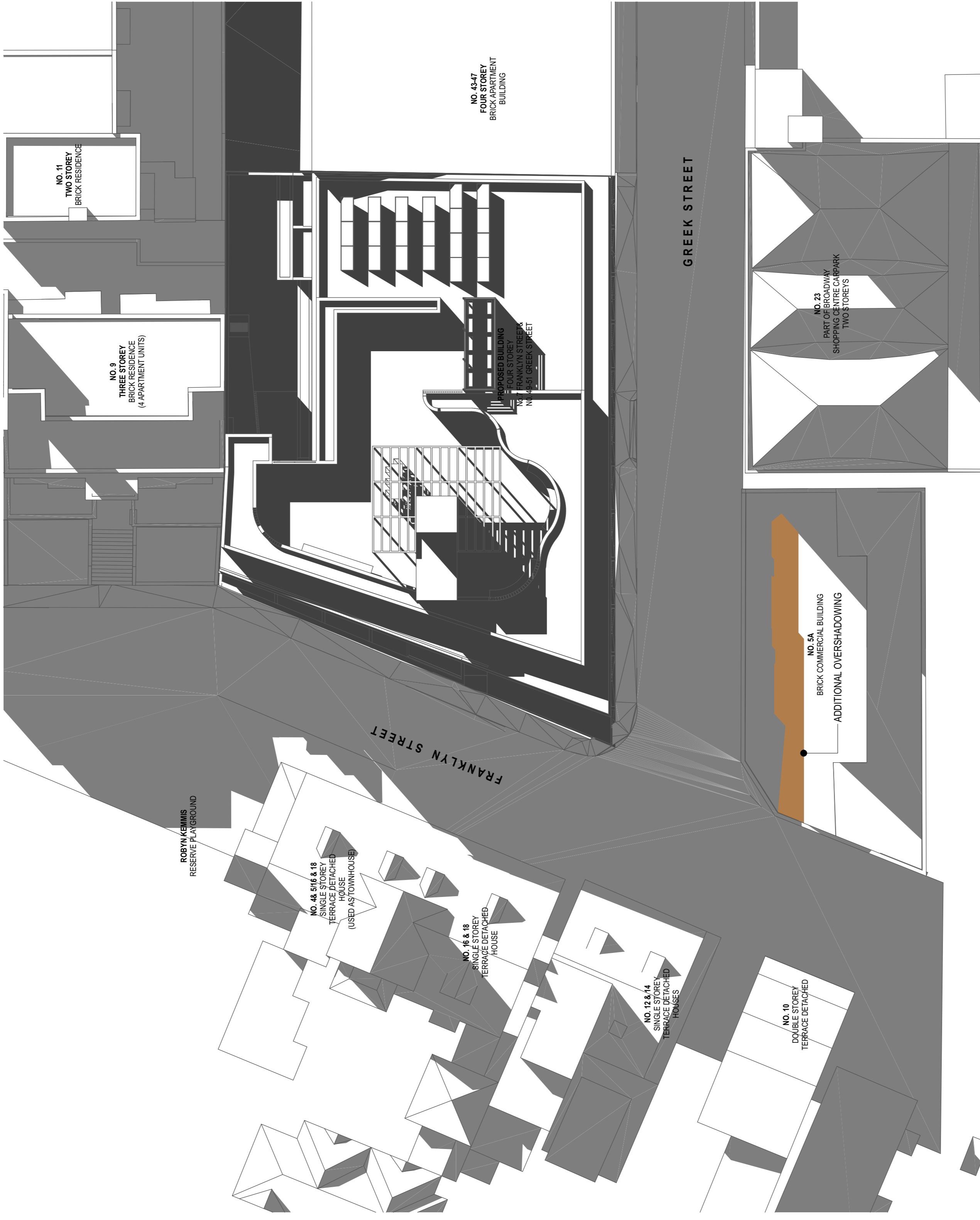
2 PROPOSED SHADOW DIAGRAM 21st JUNE 9AM 1:200
